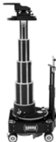
Steering Column and Tracking Bar in high position.
