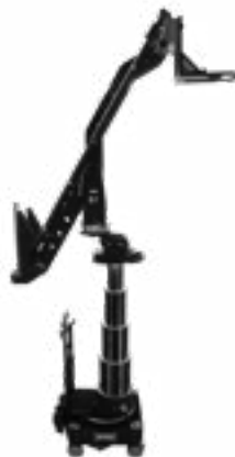
The Mitchell Head may be under-slung or over-slung.
