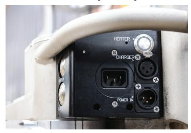
3 charging methods – 110 AC, 220 AC, and built in lithium battery – different plug for each voltage.
