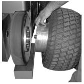
Place the solid tire on a ramp. Apply Brake. Chock opposite wheels.
