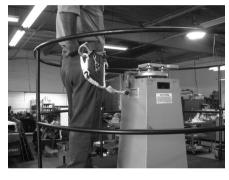
The final step in assembling the platform is attaching the safety harness. Every person on the platform MUST be attached to the pedestal with a safety harness. Even with the railing in place.
