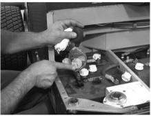
Use a hydrometer to check the specific gravity of each cell.
