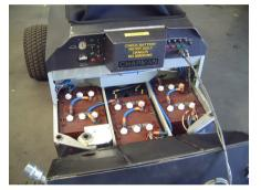
The batteries are located under the deck, in front of the driver. Lift the panels out of the way to check on their condition daily.
