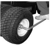
**Torque** the Center Hub Bolt to 220-250 lb. (The Lock Washer should now be completely flattened).
