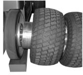
While holding a Knobby Tire up agains the Solid Tire, **Align** the Five Lug Nuts on the Solid Tire with the Five Holes on the Knobby Wheel.
