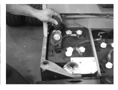
Use a hydrometer to check every cell in the batteries before using the Olympian III.
