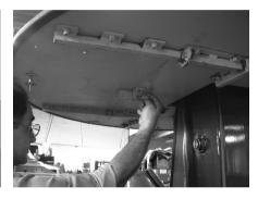
A quick release pin secures the section to the center section of the platform. The quick release pin used for securing the section to the pedestal may be stored in the hole next to the retaining quick release pin.
