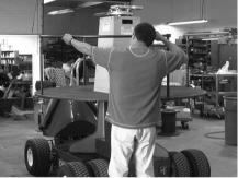
Attach the three quarter circle sections of the safety railing.
