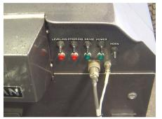
Begin by turning on the **Power**, located on the chassis in front of the drivers seat. Next switch on the **Drive** and the **Steering** controls. Then switch on the **Leveling** if necessary.
