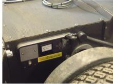
Charging and monitoring the batteries can be done at the left rear wheel of the Olympian III. Check the batteries every day and make sure that the water level in each cell remains within 1/8" from the top.
