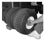
Wiggle the Knobby Tire to insure that the Lug Nuts are embedded in the Five Holes. Hold the Knobby Tire against the Solid Tire by wedging your foot under the Knobby Tire. Tighten by Hand.
