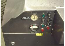
You may choose to **manually level** the center post using switches on the left side of the control panel.
