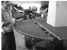
Align the support struts to the center section of the platform and slide into place.
