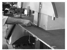
The center section of the platform is already mounted on the Olympian III when it arrives on the set. The two side pieces that complete the platform's circle are attached by a quick release pin on each side of the pedestal. The struts fit into recesses in the main platform deck to secure it in place and provide the Olympian III a narrow profile during transport.
