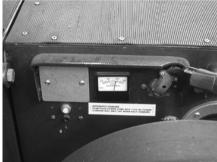
Charge the Olympian III overnight. A gauge located on the left rear of the chassis shows the rate of charging.
