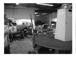
Attach the four single rods around the platform to begin building the safety railing.
