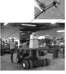
The fourth quarter section of the safety railing is placed to the rear of the Olympian III. It has a quick release pin at one end to allow the cameraman to mount the platform without having to climb over the railing.
