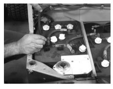
Top off each cell to within an eighth of an inch from the top of the neck using **DISTILLED WATER (ONLY).**
