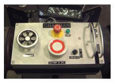
The Steering Control, Emergency Stop, Raise/ Lower Center Post, Power switch for Automatic Leveling, and Forward and Reverse Movement of the vehicle can all be accessed from the Driver's seat.
