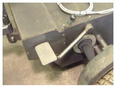
Two **Brake** pedals can be reached from the driver's seat on the Olympian III. They may also be locked in place by pushing down on the **Brake Lock** knob.
