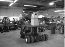
When the safety railing is securely in place, the cameraman can climb onto the platform by detaching the lower railing at the quick release pin. Be sure that the quick release pin is reattached securely.
