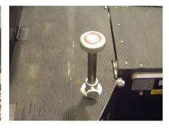
The center post column can be raised and lowered by turning the Control Handle at the left rear of the Olympian III.
