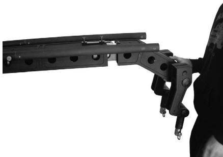
Replace the Nose on the end of the Arm.
