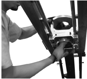
Separate the Mitchell Mount Head from the Glider Mechanism.
