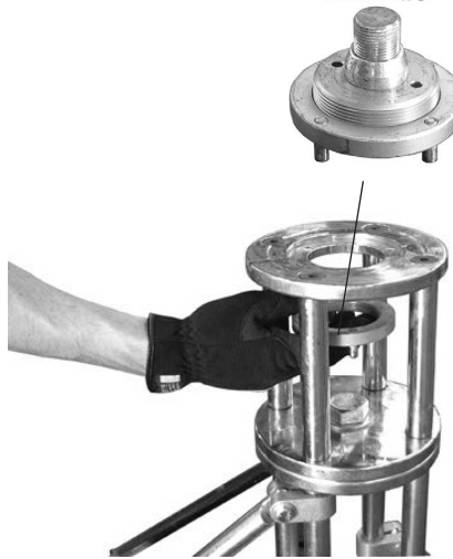
High Post Adapter installed and ready for the Stinger™ Jib Arm to be mounted.
