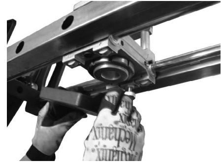
To change to the Underslung Mode, first remove the rubber cover from the Gliding Head.
