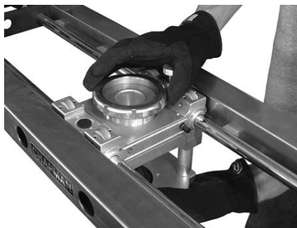
Attach the locking ring to the Mitchell Mount Head.
