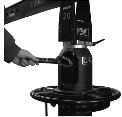
Use the special Castle Ring Wrench to tighten the Castle Ring.
