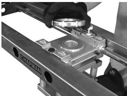
Raise the Mitchell Mount Head until its threads become visible above the Glider Mechanism.
