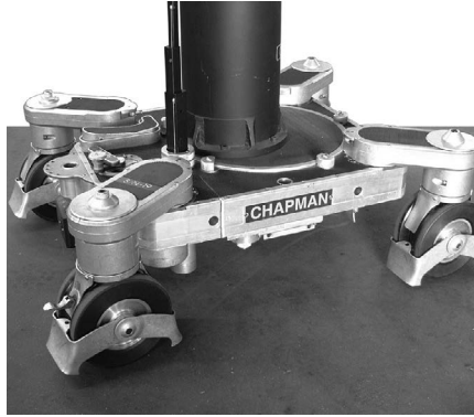
Before mounting the Stinger™ Jib Arm on the Center Post Insert, all legs MUST be in the 45 degree configuration. This will provide maximum stability for the base.
